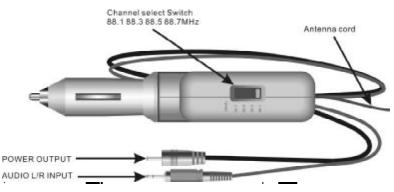
This power adapter has a built-in wireless FM Modulator. The FM modulator is designed to transmit the audio from your DVD player to your vehicle radio.
